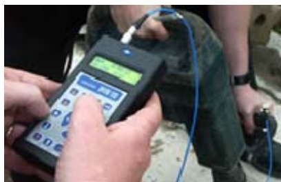
Measuring hand-arm vibration levels with a datalogger
